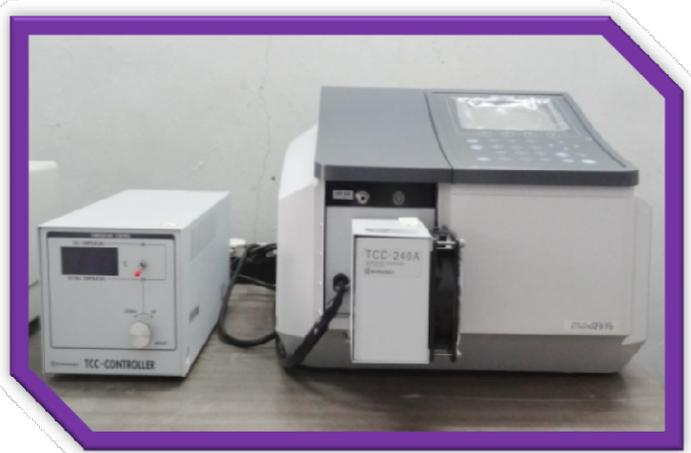
**UV-VIS Spectrophotometer; Toshwin, Rs 7.0L**
