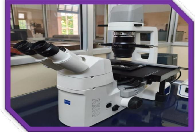
**Fluorescence Inverted Microscope; Carl Zeiss; Rs 14.0L**
